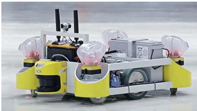
At Magna factories, the parts used in car interiors and exteriors are transported from the warehouse to the robot by autonomous transportation systems.
